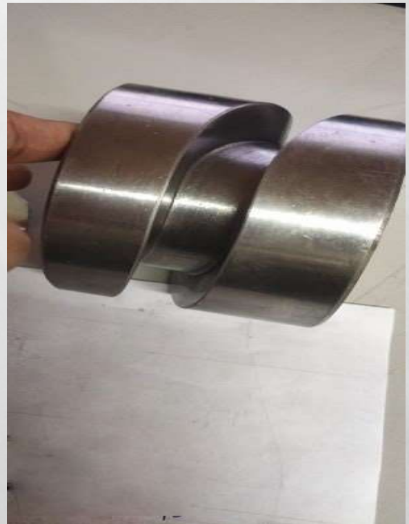
Development of a Special Cam on 5 Axis CNC Milling Machine
